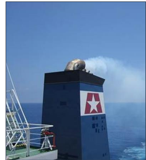
During commissioning of the vessel scrubber in operation
